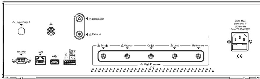
Fig. 2-2 Basic Structure of ADT780 rear panel
