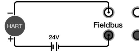
Figure 17 HART external power / internal resistance
