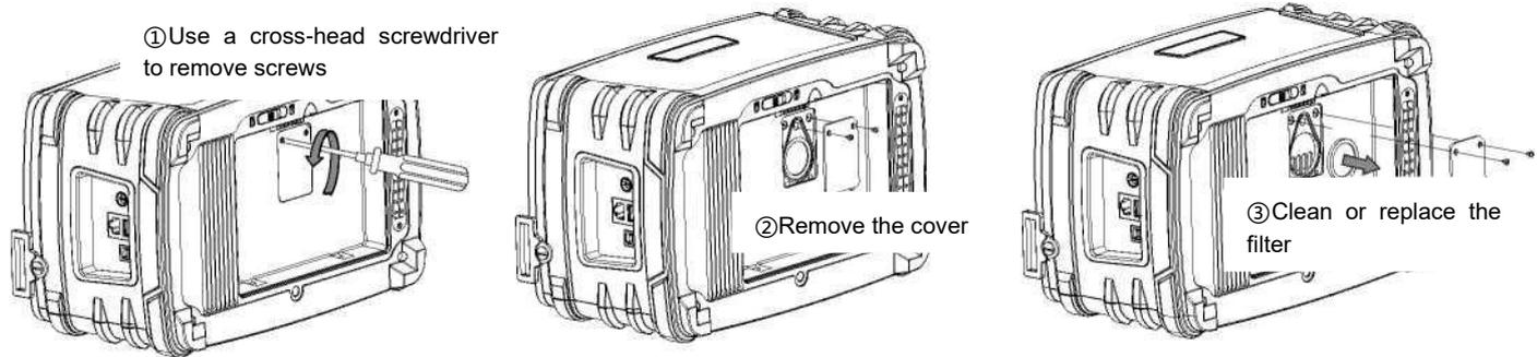
Figure 8- 1 Disassembly of the suction filter
