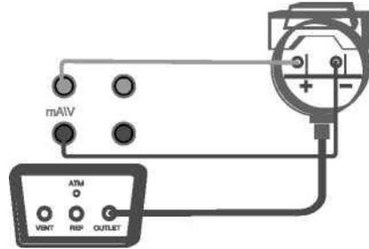
Figure 3- 13 Calibration of a 2-wire pressure transmitter
