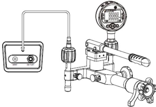
Figure 4- 1 Calibrate an barometric pressure module
