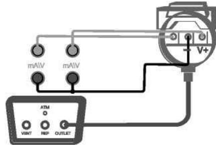
Figure 3- 14 Calibration of a 3-wire pressure transmitter
