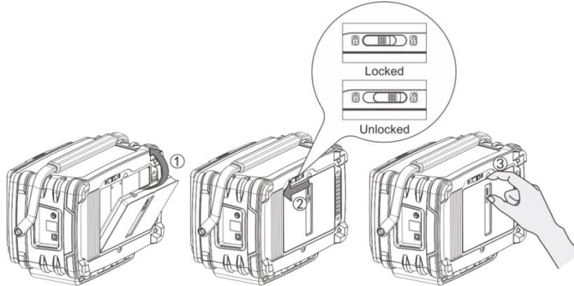
Figure 2- 3 Battery installation
