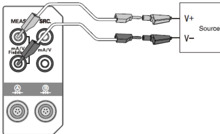
Figure 3- 6 Voltage measurement
