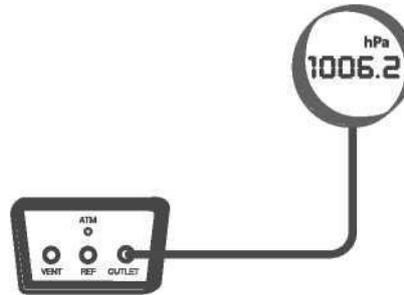
Figure 5- 6 Calibration of the general digital barometer
