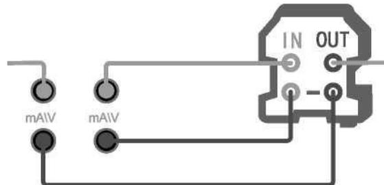
Figure 5- 3 Calibration of the signal isolator
