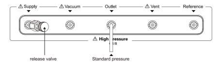
Fig 7-1 Connection of External Standard Pressure
