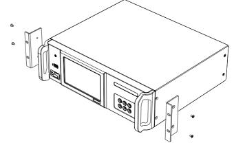
Fig. 3-1 Rack enclosure installation diagram
