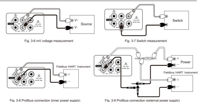
Profibus /HART® supports connection using internal loop power and external loop power. When the external power supply connection method is adopted, a  $250\Omega$  electric resistor shall be connected additionally.
