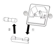
Figure 7-3 Diagram of Fuse Replacement
