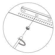
Figure 7-4 Diagram of Filter Replacement
