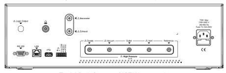
Fig. 2-2 Basic Structure of ADT780 rear panel
