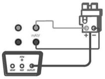
Figure 3- 17 Calibration of an I/P converter
