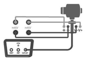
Figure 5- 2 Calibration of the pressure sensor
