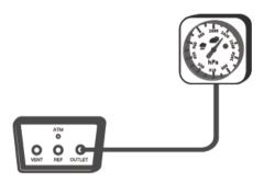
Figure 5- 9 Calibration of the aneroid barometer
