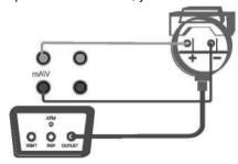
Figure 3- 13 Calibration of a 2-wire pressure transmitter
