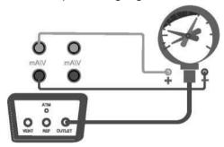
Figure 5- 4 Calibration of the contact pressure gauge
