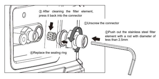
Figure 8-3 Disassembly of differential pressure connector
