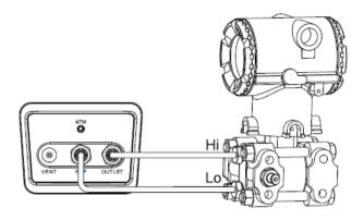
Figure 2- 6 Low pressure and differential pressure connection
