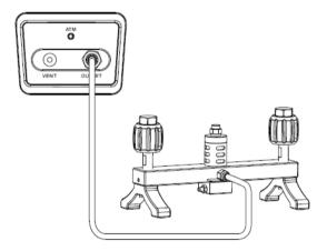
Figure 2- 5 Gauge pressure connection
