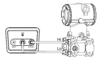
Figure 3- 2 Differential pressure outlet
