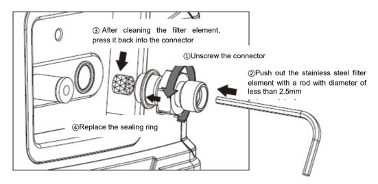
Figure 8- 2 Disassembly of high-precision/barometric (BP) version pressure connector
