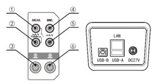
Figure 2-2 Electrical and signal port
