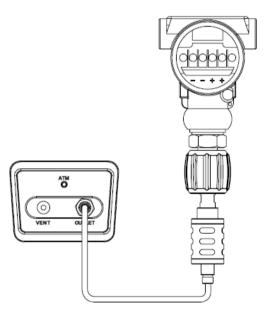
Figure 3- 3 Gauge pressure outlet
