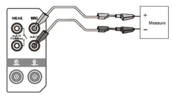
Figure 3- 10 Current output of internal power supply
