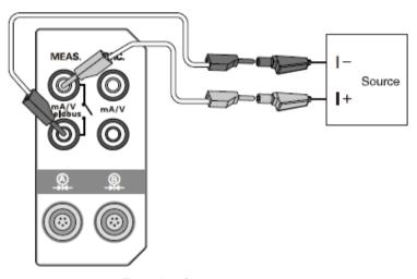
Figure 3-5 Current measurement
