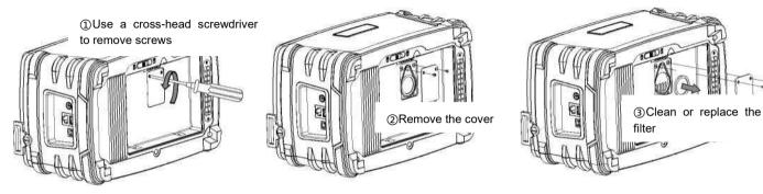
Figure 8- 1 Disassembly of the suction filter
