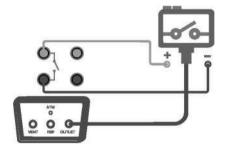
Figure 3- 16 Calibration of a pressure switch
