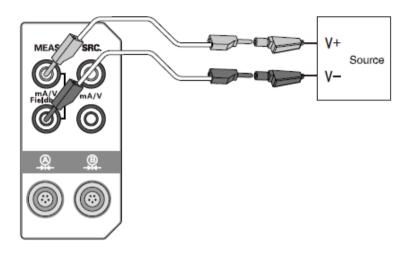
Figure 3- 6 Voltage measurement
