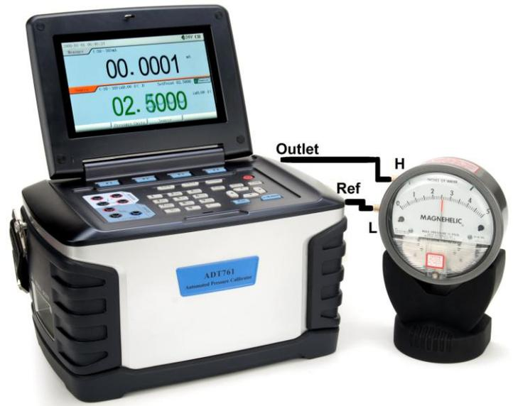
Figure 4 ADT761 calibrator with DUT
